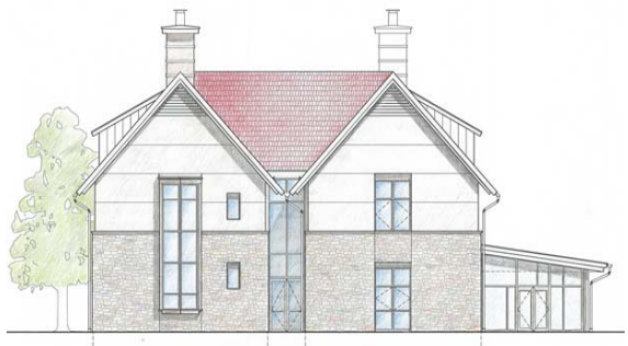
Figure 2 -Elevation of Stone & Stucco veneer by Lilley Dadagian Architects
